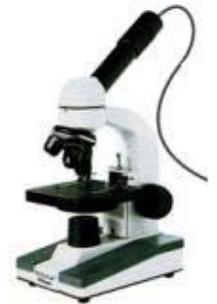
A conventional microscope can become a digital microscope quite simply with the addition of a digital eye-piece. A digital eye-piece is a special digital camera that replaces the standard eye piece of the microscope and is attached to a computer.
